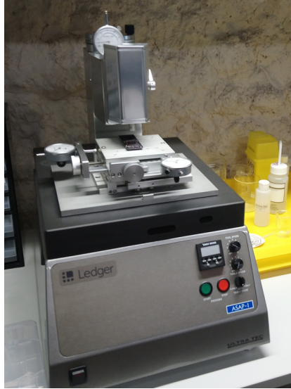
Fig. 2. ASAP1 micro-milling machine for chip decapping
