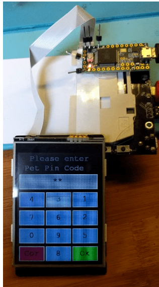
Fig. 4. WooKey instrumentation with a Teensy for PetPIN bruteforce
